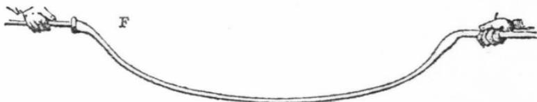
workmen are continually rotating. Some parts are cooled by fanning with the hat of an attendant boy, to ensure uniform elongation, till the cane or tube is drawn to a length, sometimes of from sixty to seventy feet: as the metal cools, the tube ceases to rotate, and it assumes, by continued tension, nearly a straight line, G; except at the extreme ends, it is
